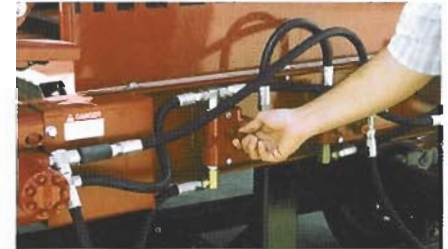
Two Hydraulic Orbit Motors with Two Manual Adjusted Flow Controls
