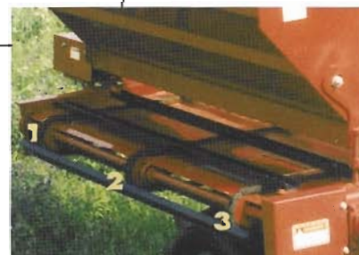
Maximum feeding three chain drive on slats
